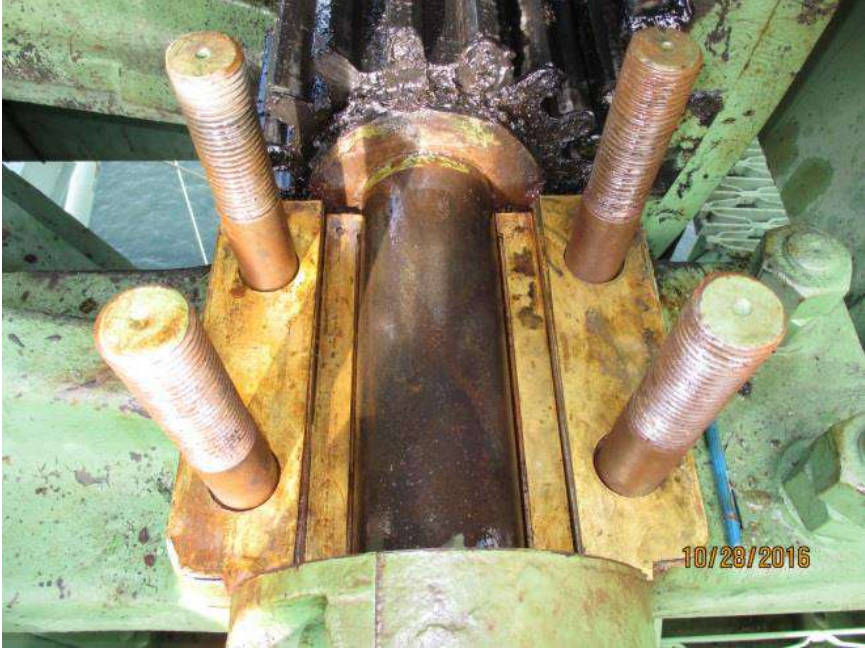
Figure 19: Northwest rack pinion bearing after cleaning.
