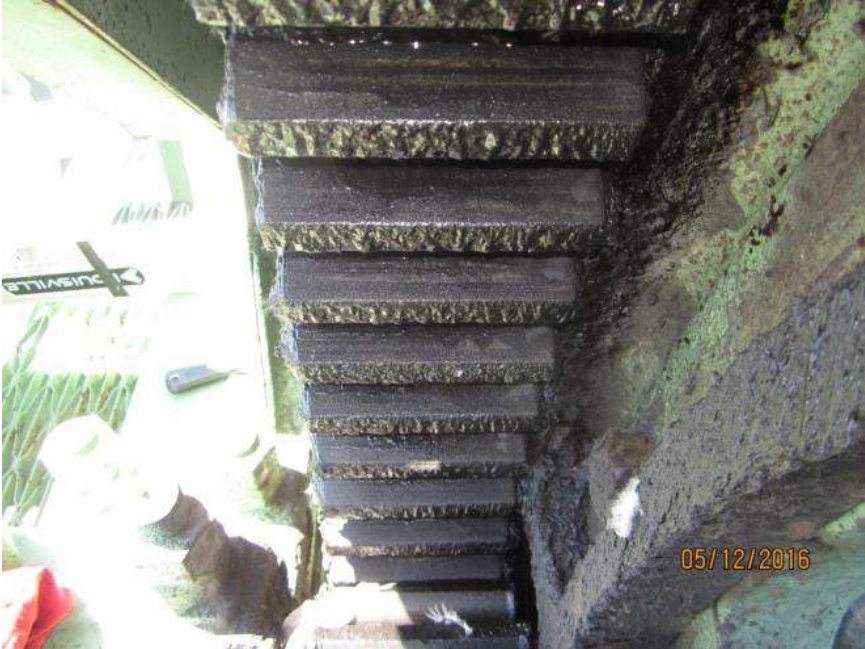
Figure 4: Rack teeth lube pattern
