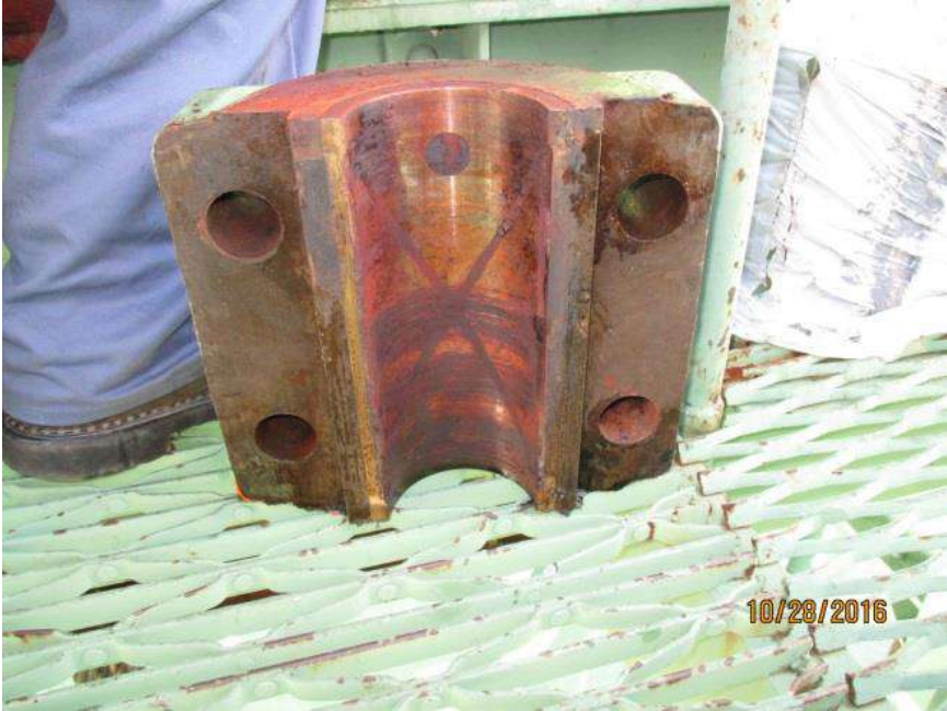
Figure 20: Northwest rack pinion bearing cap. Note clogged lubrication port and lubrication grooves
