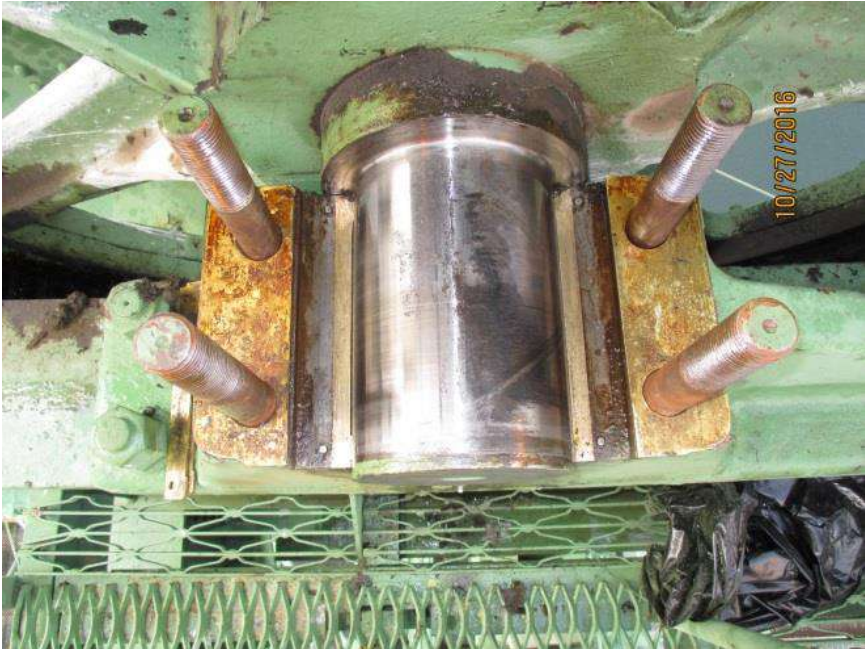
Figure 15: Typical bottom half of trunnion bearing journal.
