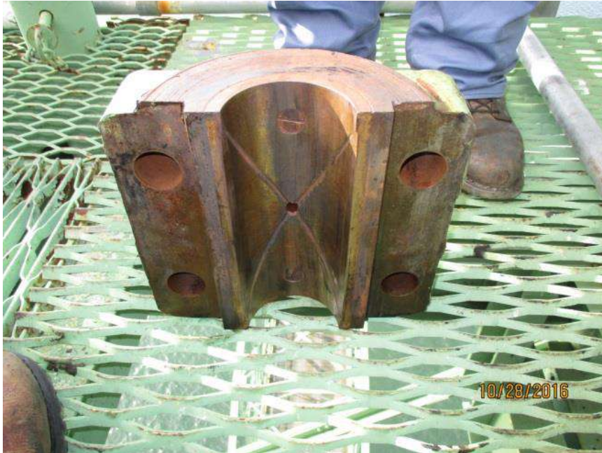
Figure 21: Northwest rack pinion bearing cap after cleaning.
