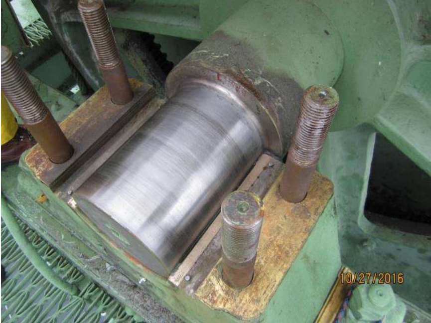
Figure 14: Typical top half of trunnion bearing journal.
