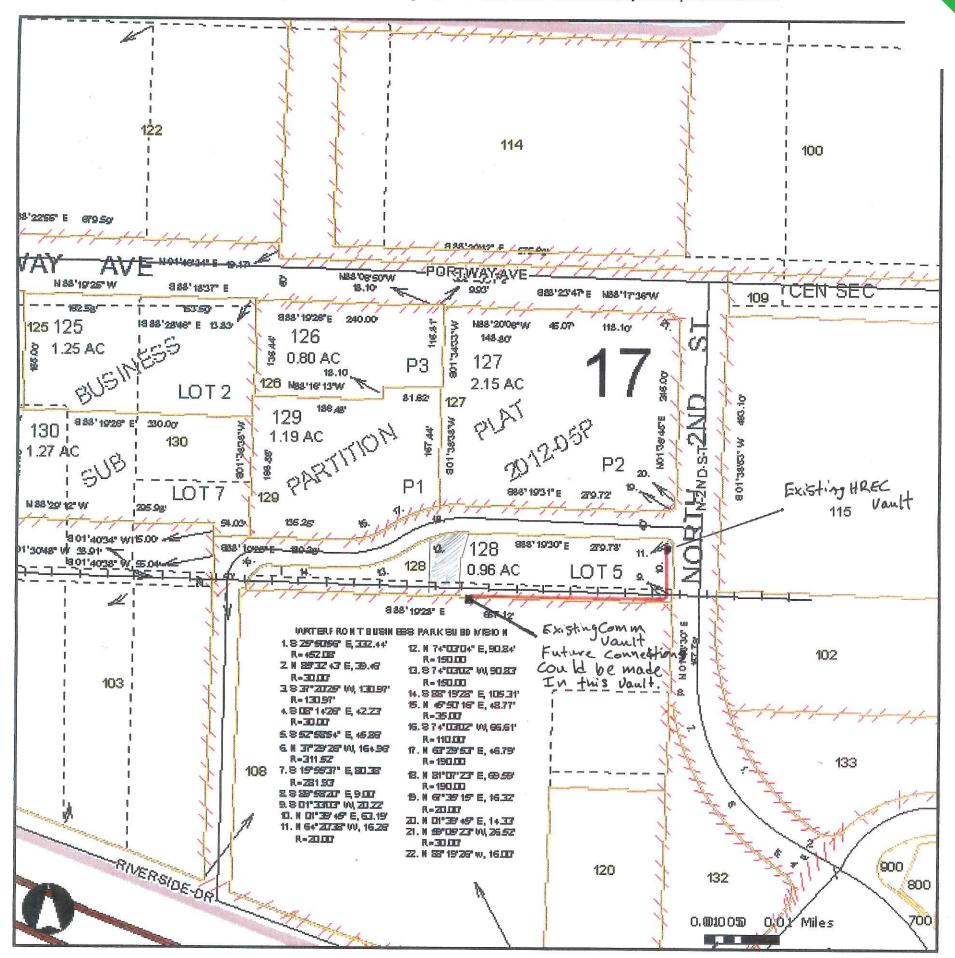
Propose 2- 2 inch conduits (one for Ryan's Juice and one for future development) from Existing HREC vault at the intersection of North 2<sup>nd</sup> and Anchor Way approximately 90 feet south then turning west for approximately 300 feet to existing Ryan's communication distribution vault.) Trench will be a minimum of 30 inches deep and all excavation shall be returned as found. Impact on existing landscaping and hard surfaces will be minimal.
