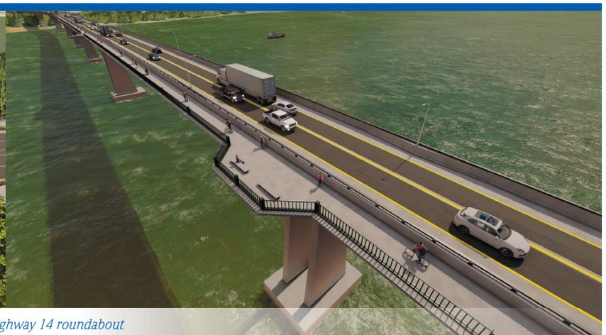
Conceptual design renderings of new bridge and Highway 14 roundabout
