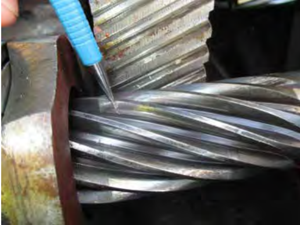
Photo 13. South Primary Reducer. View of west first reduction gear set, opening face of pinion teeth. Note the pits on the outboard (left) end of the teeth.
