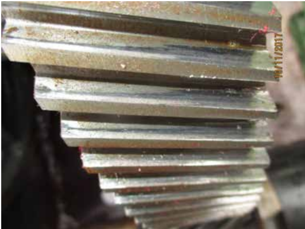
Photo 8. North Primary Reducer. View of west first reduction gear set, closing face of gear teeth. Note the heavier contact and light wear on the west (right) ends of the teeth.
