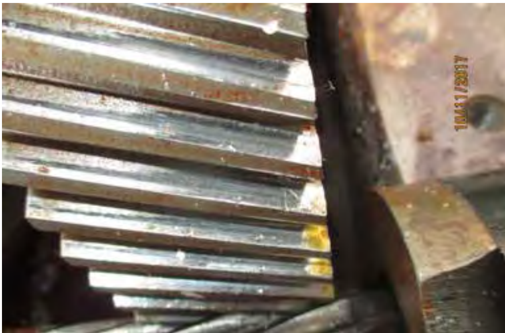
Photo 10. North Primary Reducer. View of west first reduction gear set, closing face of gear teeth. Note the damage on the west (right) ends of the teeth, presumably from particles passing through the mesh.
