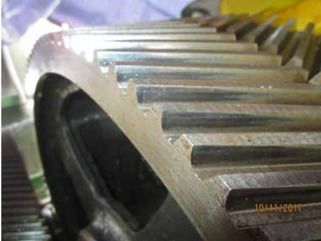
Photo 11. North Primary Reducer. View of west second reduction gear, opening face. Note the contact is 40% to 50% across the width of the teeth, starting at the west (left) end.
