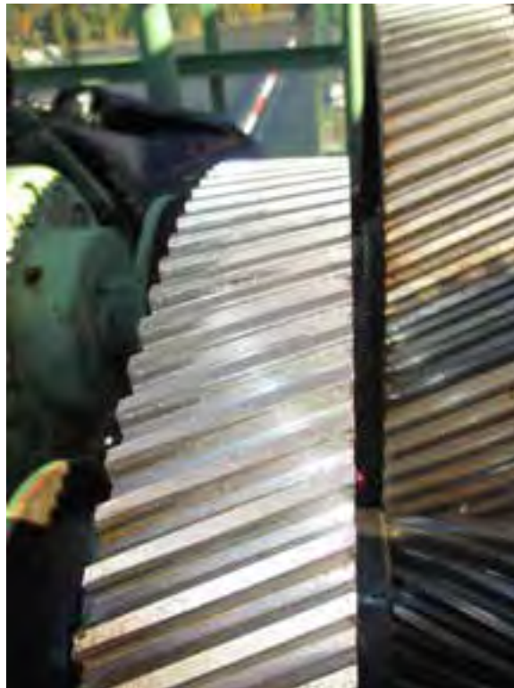
Photo 16. South Primary Reducer. View of west first reduction gear set, opening face of gear teeth. Note light pitting on the outboard (left) ends of the teeth.
